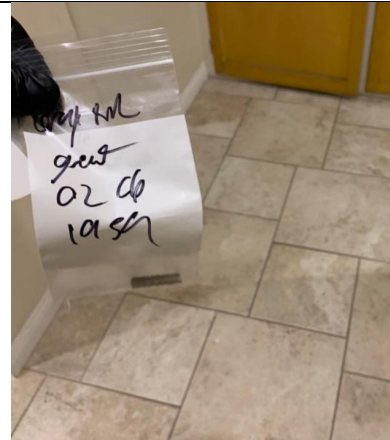
Photo of HA number 19, Sample No. 0206-19-59 | Non-ACM Gray Tile Grout, Within Hallway and Kitchen
