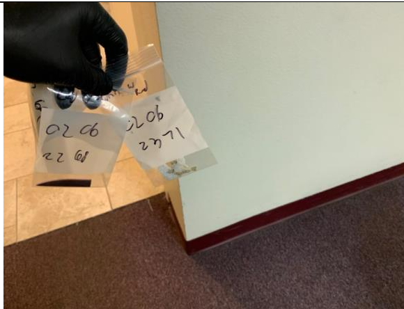
Photo of HA number 22 & 23, Sample No. 0130-17-51 | Non-ACM Red 4" Cove Base and White / Red 4" Cove Base Associated with Mastic, Within Open Room, Day Room and Bedroom 1
